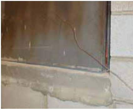
6. Door warped from heat during test
